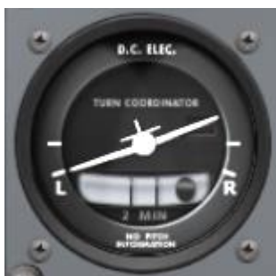
Aircraft skidding to inside of turn
