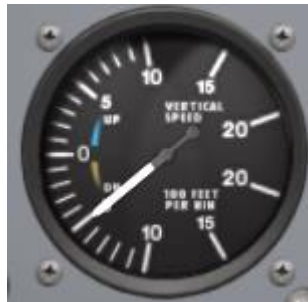
Aircraft descending -500ft/min
