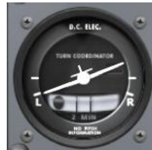
Aircraft slipping to outside of turn
